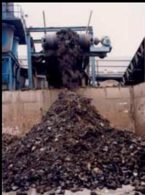
Everything including the kitchen sink! This shows the diversity of the scrap pile that the End of Life Vehicles join for recycling aimed at the recovery of metals. Large recoverable plastic parts and pollutants having been removed prior to this stage.
